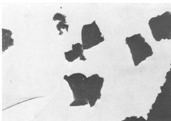
Fig. 3. Electron micrograph of a sample of montmorillonite after heating at 1000 °C; magnification 7000 ×
